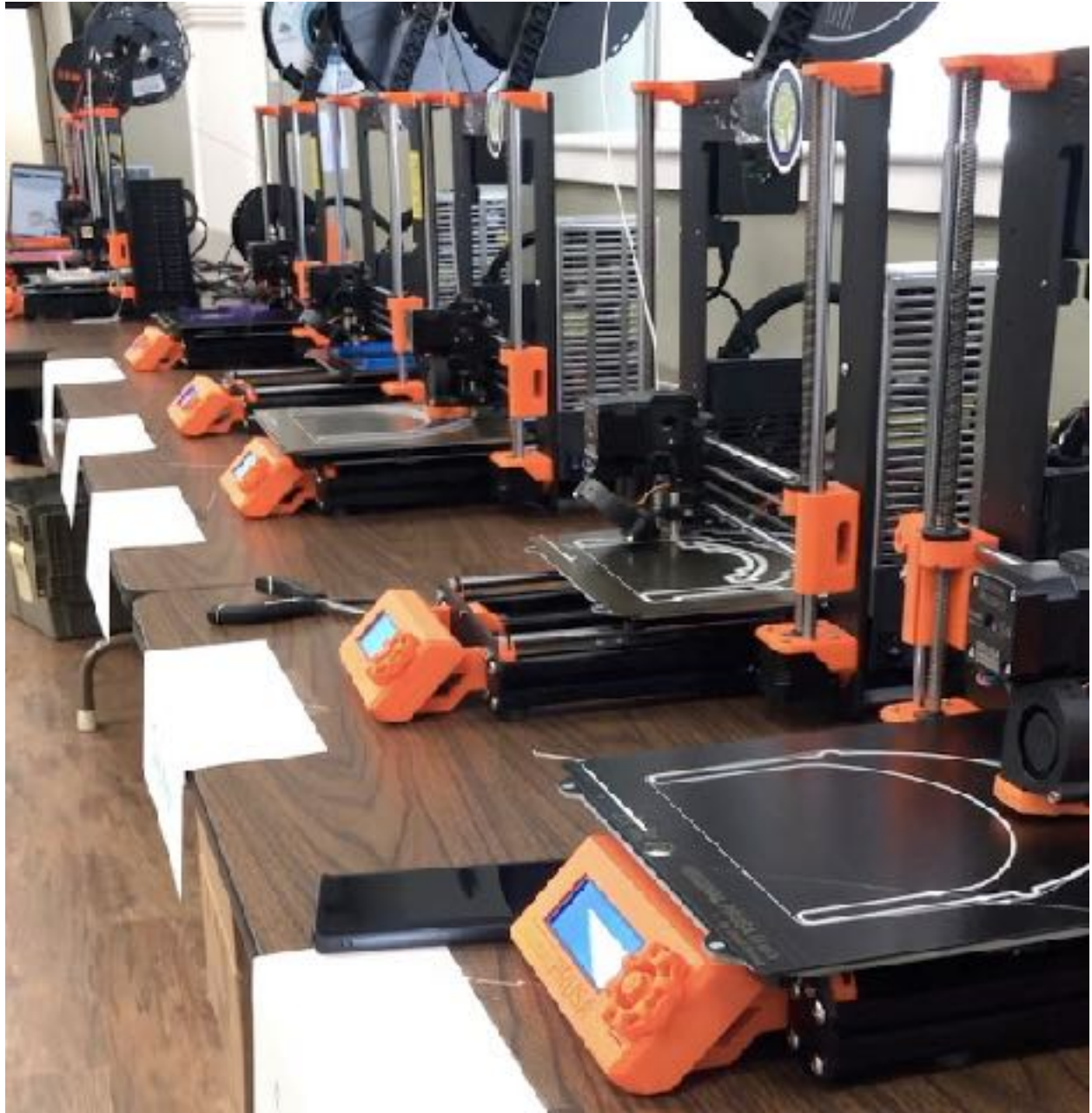
Face shield parts being 3-D printed at the Suffolk Cooperative Library System
